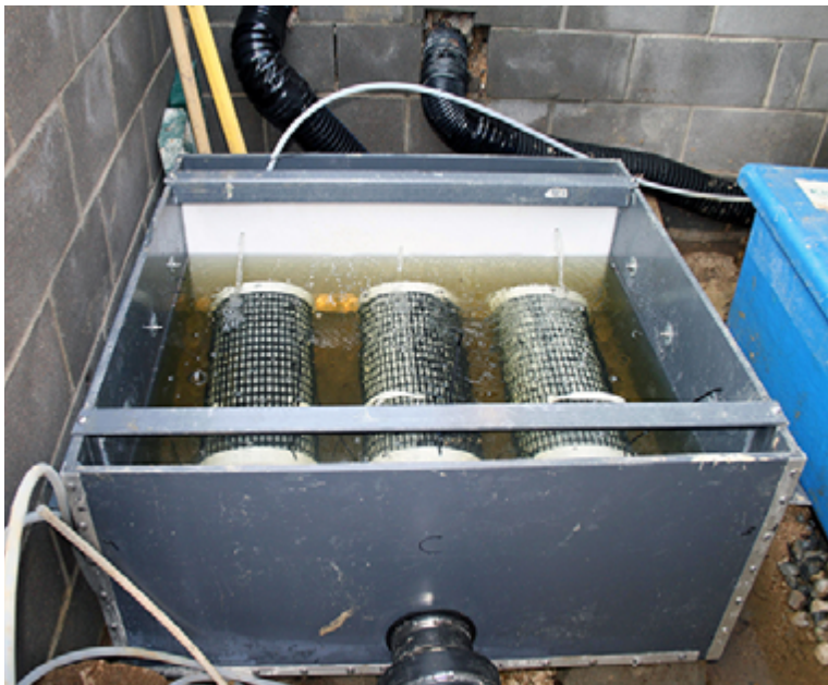
Various filter materials are being tested for their efficacy to remove nutrients (N and P) and pesticides (chlorothalonil, mefenoxam, and propiconazole) from drain lines before leachate is discharged into surrounding surface water.
