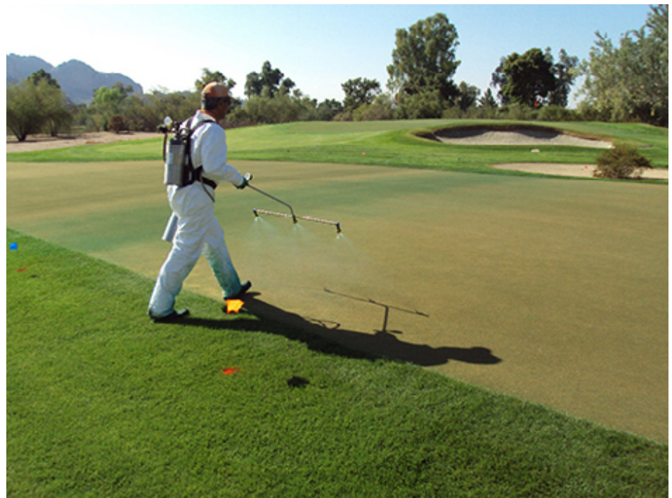
Colorants were applied using a CO 2 -powered backpack sprayer with a hand-held three-nozzle boom with TwinJet™ 8008 flat fan nozzles spaced 20 inches apart.
