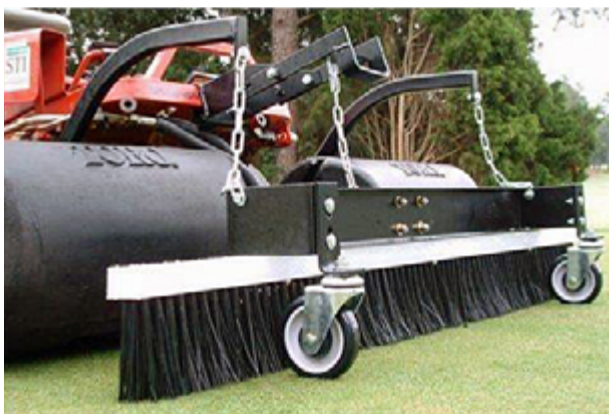
Turf managers who use riding greens mowers are not without options. Some manufacturers offer brushes designed for their mowers, and the brush pictured here can be equipped on most John Deere, Jacobsen, or Toro models.
