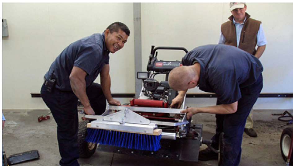
This front-mounted brush is 2.5 times as deep as currently available models. It can be mounted on some John Deere and Toro walking greens mowers. This brush can be easily adjusted to increase or decrease the impact it has on the turf.
