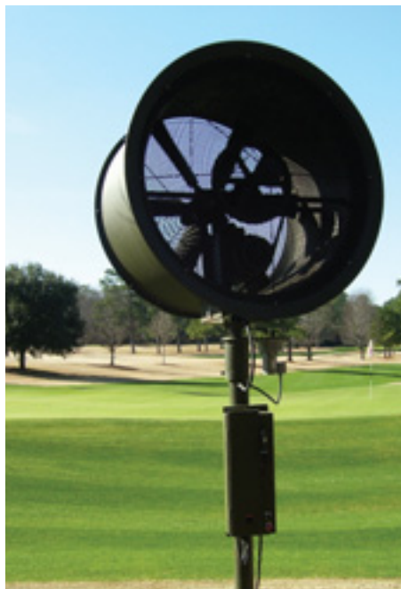
Above left: A combination motor starter and disconnect switch is installed on the upper fan pole on this three-phase motor fan. Since three-phase motors don't have thermal protection, it is essential to install these devices to protect the fan motor. Above right: Concrete is used to secure the four-foot ground pole that attaches to the fan pole. The concrete provides a long-term stable foundation for the fan.
