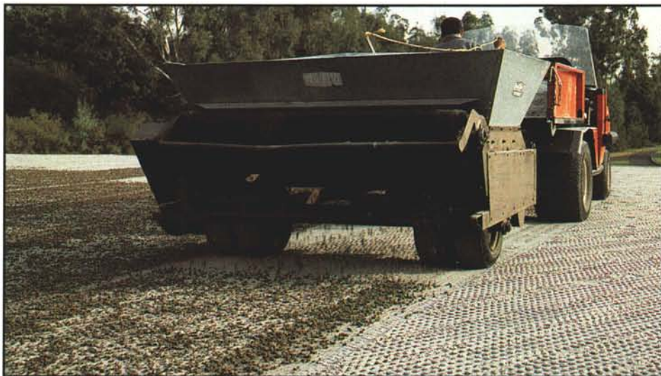
A mechanical topdresser is used to spread aerification cores evenly on the surface of the nursery.
