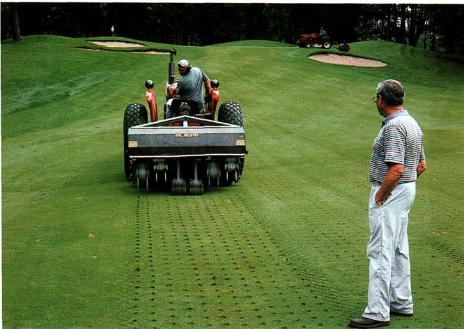
Deep-tine aeration can relieve compaction found beyond the reach of conventional core cultivation operations.
