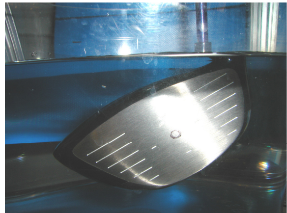
Figure 5.5 (b) – Clubhead Immersed in Container with Hosel above the Surface
