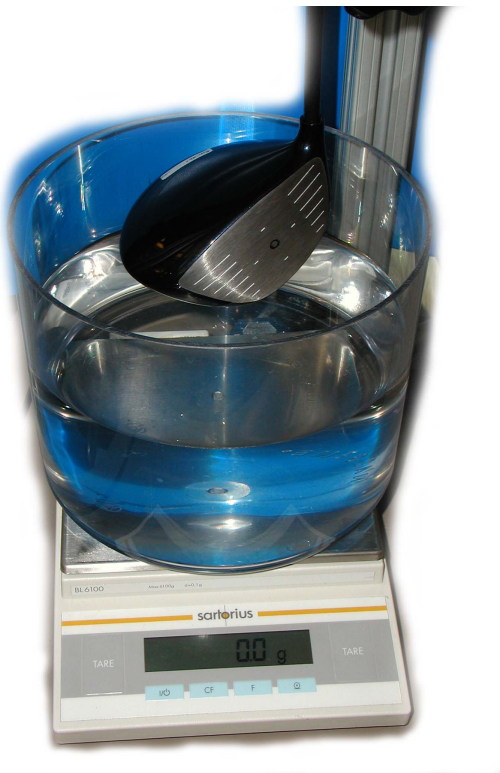
Figure 5.4 – Tared Electronic Scale with Water-Filled Container Ready of Clubhead Immersion
