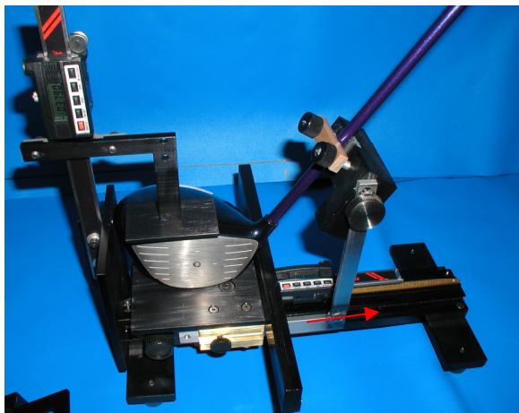
Figure 6.5 (a)–Slide Shaft Clamp Until the Heel of Clubhead Rests Against Heel Plate
