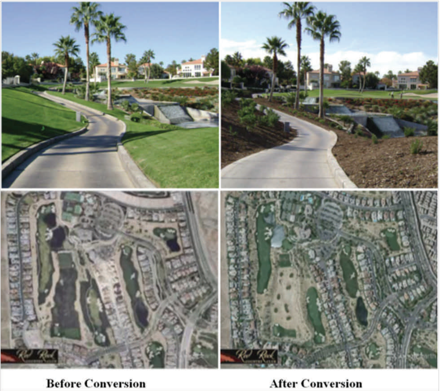
Figure 5. Examples of golf courses removing turf from out-of-play areas, perimeter areas near homes, and driving ranges. A water savings of 34 gallons per square foot was realized for areas converted from turfgrass to desert landscape.
