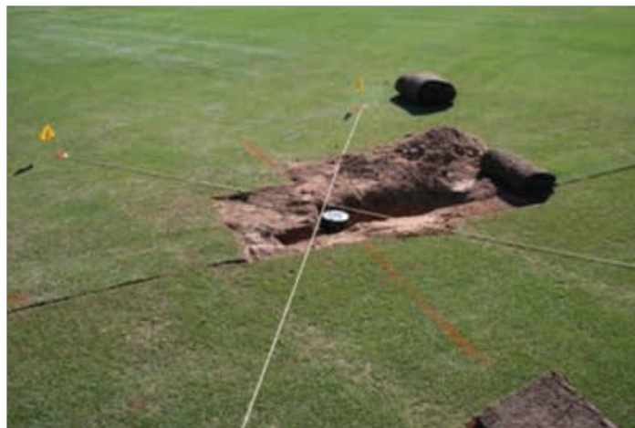
Figure 1. A mini-triangulation system was developed to protect the true location of each sprinkler in the field.
