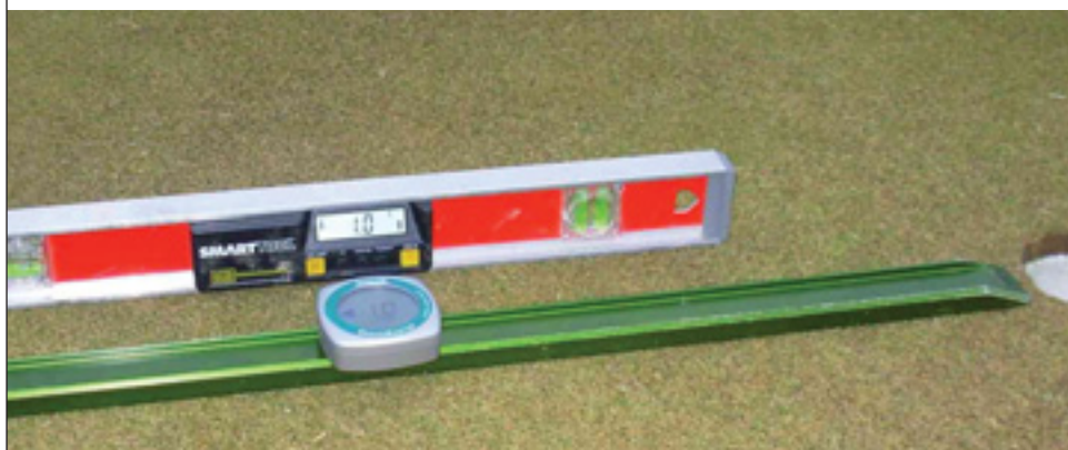
Placing digital tools on a Stimpmeter or a straight level improves accuracy.
