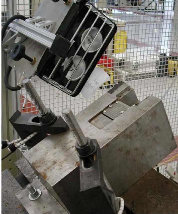
**Figure 6.2:** Grooved test plate oblique impact test setup
